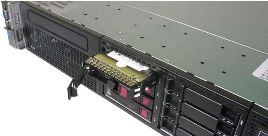
Figure 14 Pull disk latch to remove hard drive for Infoblox 4000 Series
